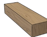
Wooden block (to plaster cement onto the brick structure).
